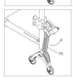
• Once the wheels are fitted, you can return the anti-tippers to their starting position. To do this, push the wheelchair forwards and at the same time push back the holding rod [73] using your foot.
